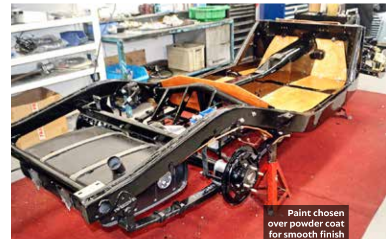
MGB disc brakes in place of MGA's drums
